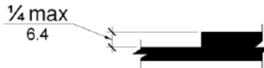
Figure 303.2 Vertical Change in Level
