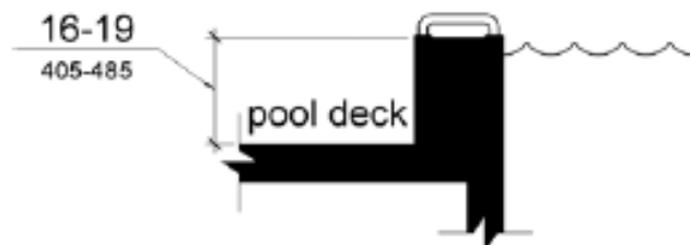
Figure 1009.4.2 Transfer Wall Height
